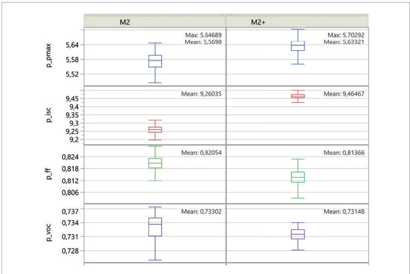
Figure 3. Results of larger-area wafer (M2+) implementation.
