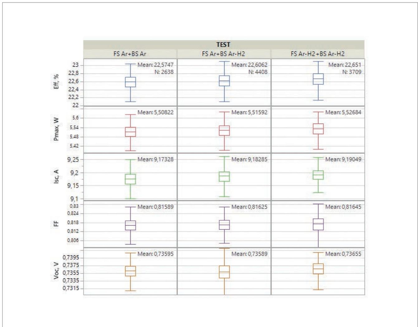
**Figure 4. Results of ITO layer optimization by adding an Ar/H<sub>2</sub> mixture during magnetron sputtering.**
